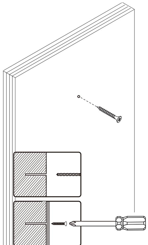
**EN** If it is a solid wall, please use expansion and self-tapping screws, if it is a wooden wall, only use self-tapping screws, please do not overtighten the screws
