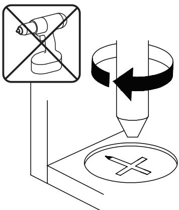
**EN**\_Turn cam lock clockwise to tighten.
