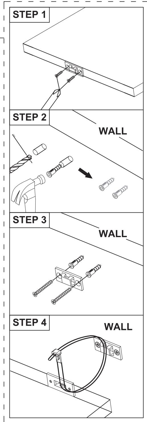
**EN** If it is a solid wall, please use expansion and self-tapping screws, if it is a wooden wall, only use self-tapping screws, please do not overtighten the screws
