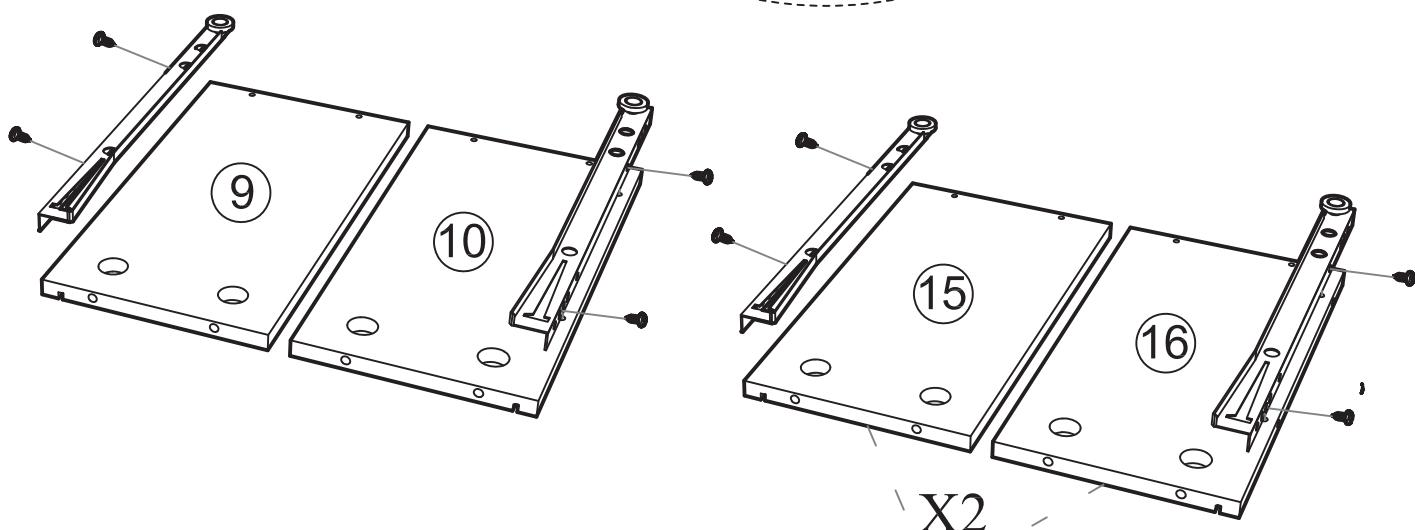
**EN** Please find the exact hole for installation, otherwise it will be misaligned. The screws on the drawer slide must be leveled , otherwise it will affect the smoothness of the drawer.
