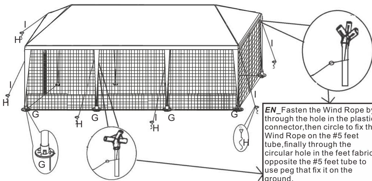
**EN\_** Fasten the Wind Rope by through the hole in the plastic connector, then circle to fix the Wind Rope on the #5 feet tube, finally through the circular hole in the feet fabric opposite the #5 feet tube to use peg that fix it on the ground.
